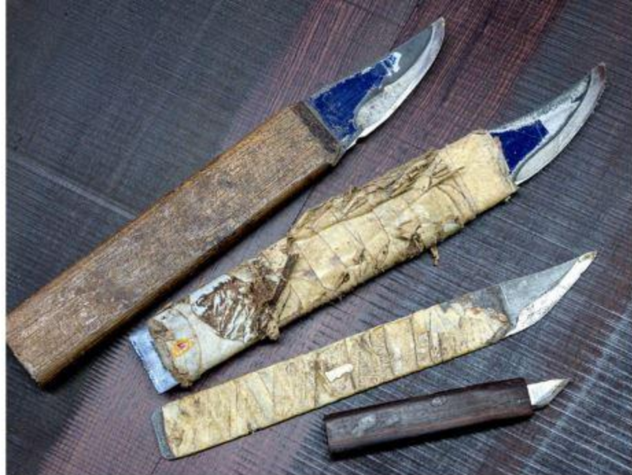
A luthier's hand-knife is often made with upcycled metal.
