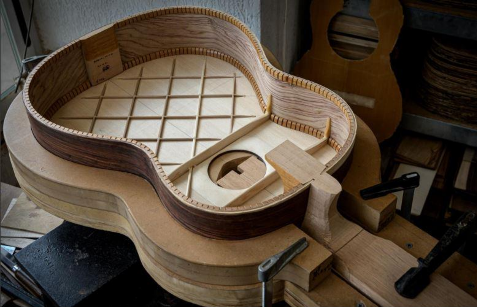
Construction of the all-wood lattice bracing.
