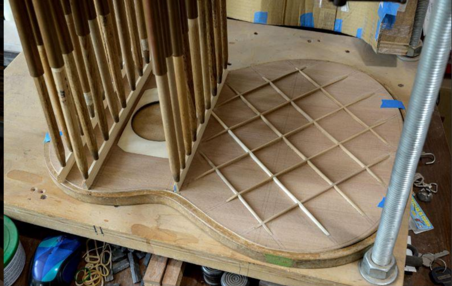
Bonding the lattice bracing to a double-top of spruce and red cedar.
