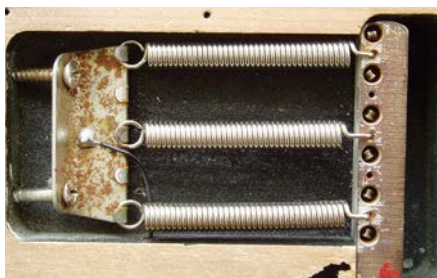
The traditional Fender Stratocaster trem system allows you to use anything for two to five springs. Here we show all the usual combinations and configurations
