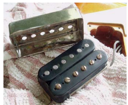
Covers are usually held in place with two blobs of solder. Use a Stanley knife to cut through the solder, being extremely careful with your fingers and the pickup itself, then lift the cover off. Here we see an 'uncovered' double black Shed PAF Daddy.
