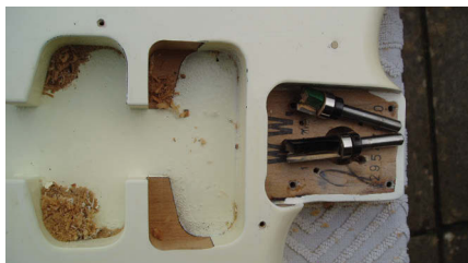
We used the same 3/8" bit for the second cut then swapped over to a 1" bit for the final cut. When we had finished, the pickup cavity was big enough to accommodate a humbucker. You can see the router bits we used in the neck pocket
