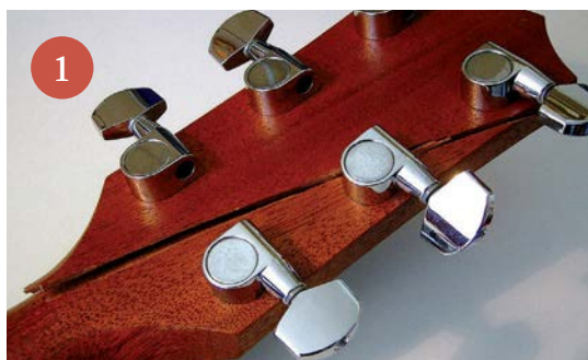
2 Over-tightening a truss rod can have expensive results
