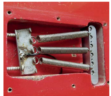
This spring claw is intentionally angled because it has been adjusted to provide precise intervals when the bar is pulled up.
