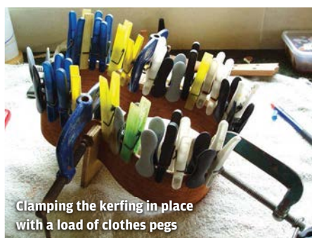
The linings or 'kerfings' come pre-bent too. Which is nice
