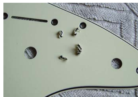
Here the volume pot hole has been widened, and we're about to move onto the tone pot hole
