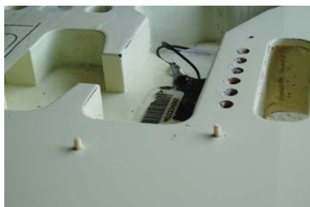
We squeezed wood glue into the screw holes and tapped in rounded-off matchsticks to plug them
