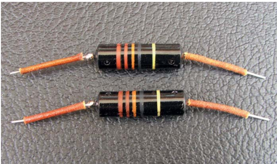
0.022uF paper/oil capacitors nicknamed 'bumblebees' were installed in original Les Pauls. Replicas are available but not all are paper/oil. Russian made K40V and K42V paper-oil capacitors are readily available cost effective equivalents.
