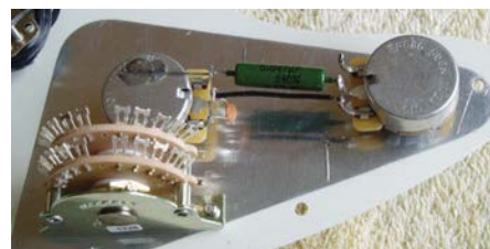
Above: the pots and Super 5-Way switch were installed and initial connections made first. Note the treble bleed capacitor on the volume pot and the way the tone capacitor is wired point-to-point
