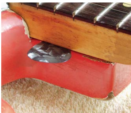
If your Strat's neck screws appear to be fully tightened but there's still a gap visible between the body and the neck, it requires some attention. Assuming there's no shim, there should be no gap whatsoever.
