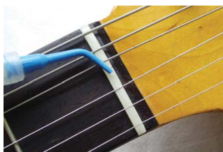
After polishing the string slots, try adding some suitable lubricant. Here we're applying some Big Bends Nut Sauce: it's good stuff
