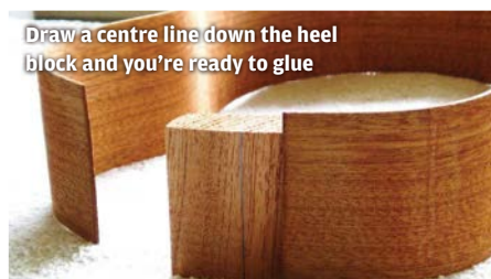
One side of the ribs are glued; now for the other side
