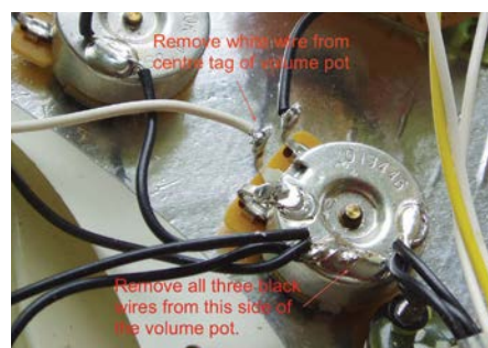
Above: these are the wires you must de-solder or snip to remove the scratchplate assembly
