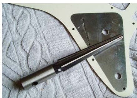
Rather than drill out the scratchplate holes to widen them for the new pots, we used a reamer
