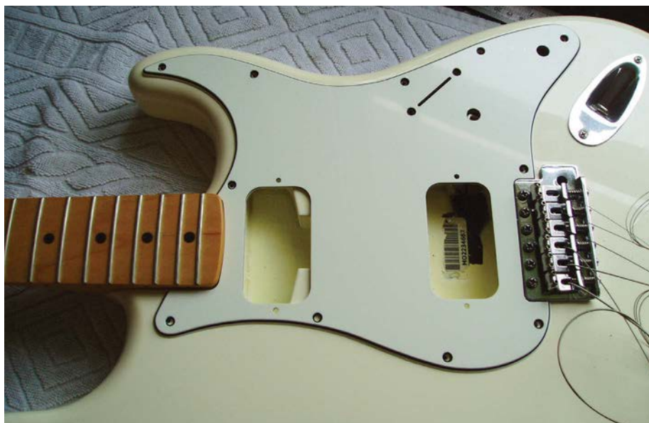
Above: the new scratchplate was a good fit but the screw holes didn't quite line up
