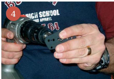
4 Adapting the flats Drilling out the holes to 5mm
