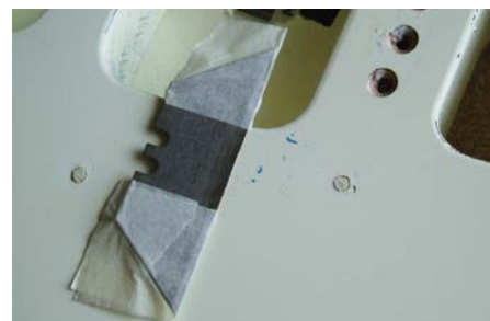
You can use a fresh blade to trim the tops of the matchstick plugs flush with the finish
