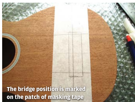
Then the excess tape is cut away. Double-check that the saddle's in the right place
