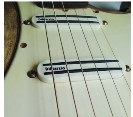
Single-coil sized dual rail pickups such as DiMarzio's Air Norton S solve hum problems and boost output, without extra routing.
