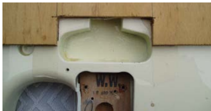
The router template might look a bit rough and ready, but the pickup cavity will be smooth
