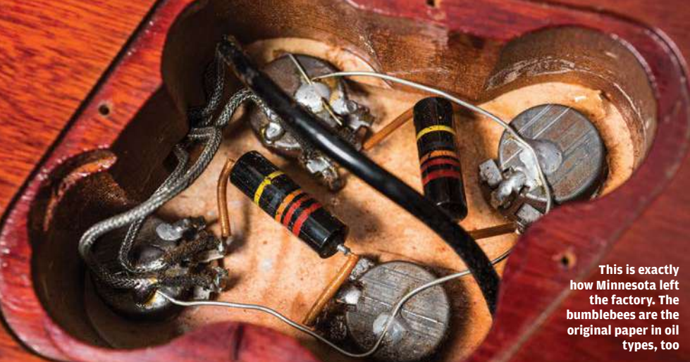
The production guitar's wiring looks very similar to the original, but the bumblebee caps are the modern mylar foil types
