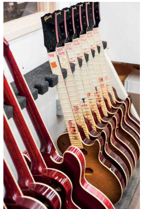
Les Pauls with their freshly glued necks clamped in place to set
