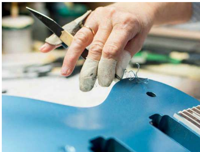
Gibson Custom's luthiers recreate the lacquer checking on a Les Paul using a razor blade
