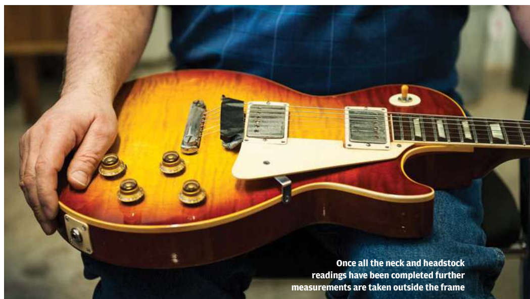
Gibson's portable scanner measures hundreds of thousands of points all over Minnesota's neck
