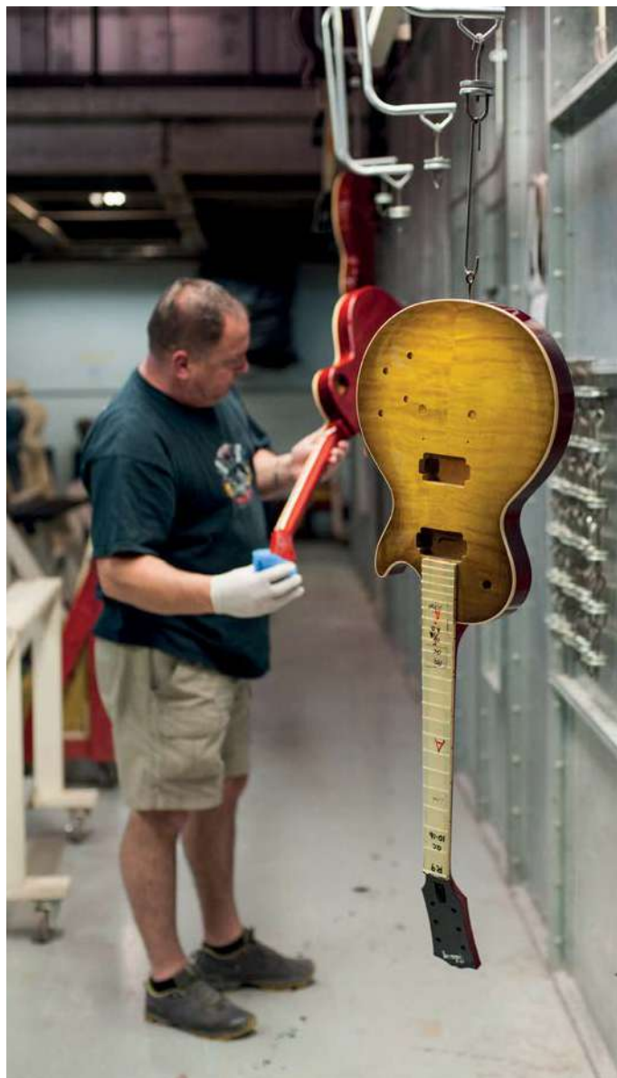
Gibson Custom's luthiers recreate the lacquer checking on a Les Paul using a razor blade
