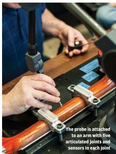
Matthew is using the slick plastic probe to scan the transition from the neck into the headstock curve
