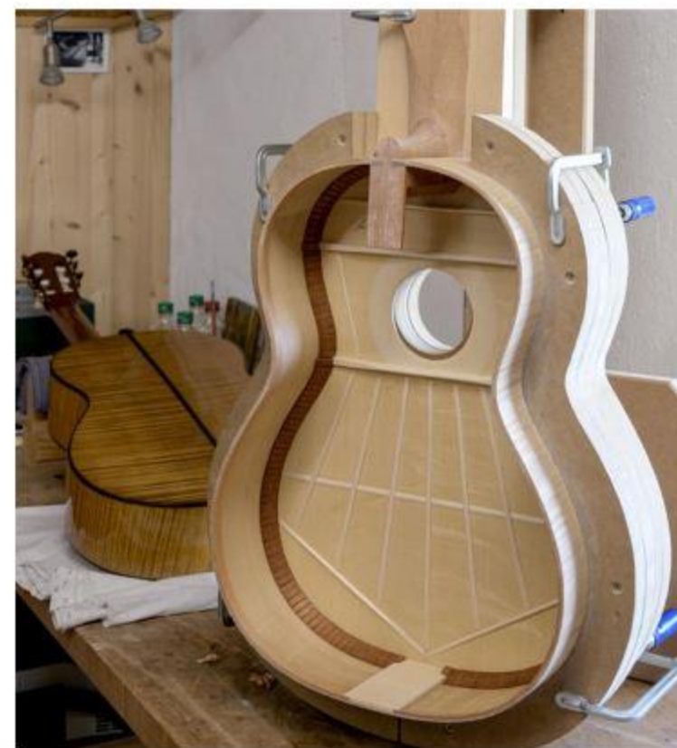
Her bracing is a symmetrical seven-strut fan, with two closing bars.
