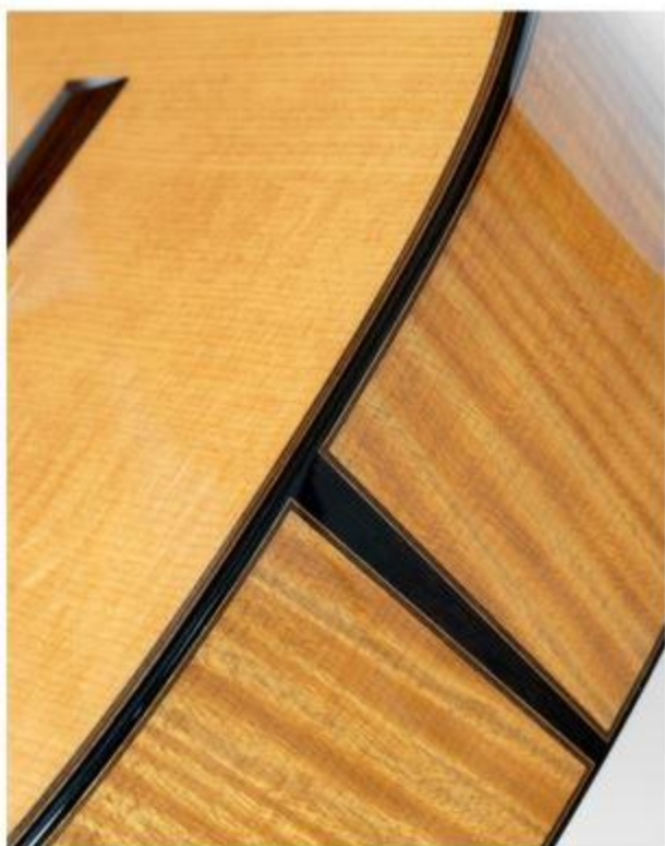
Laminated ribs and a headstock inspired by Manuel Ramírez.
