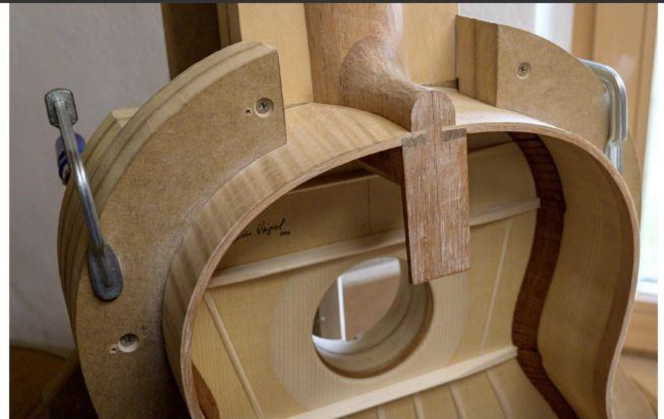
The finished heel will have a round "button", in the style of violin lutherie.
