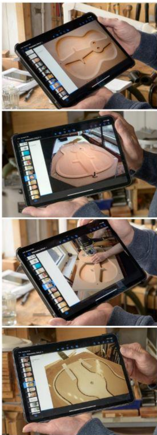
Gernot Wagner has experimented with different Nomex layout patterns in his guitars' soundboards.
