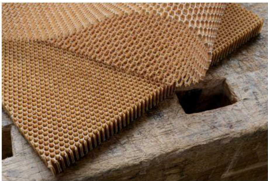
Two types of hexagonal structure: regular and elongated.
