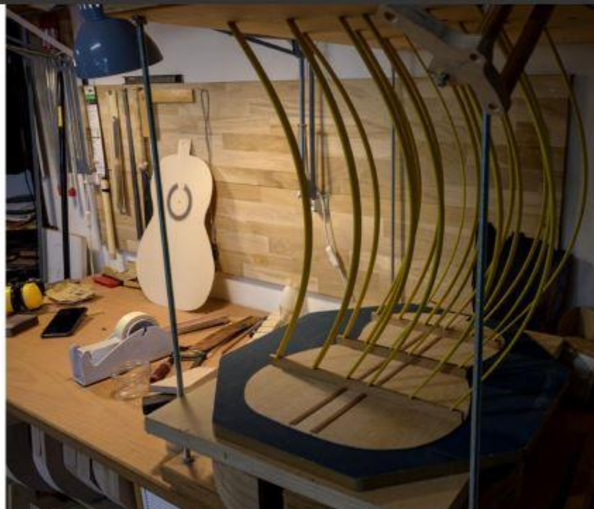
Gluing braces onto a back of maple.
