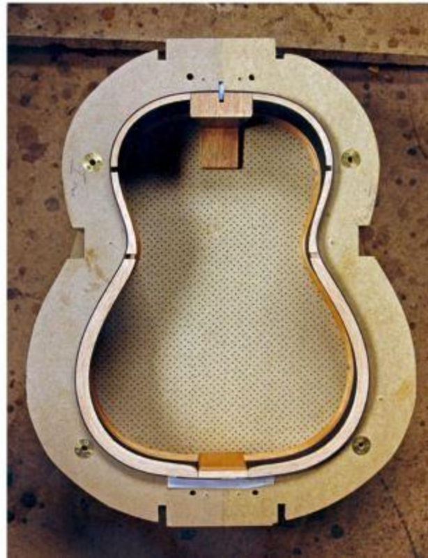
His assembly mould with ribs set in place.
