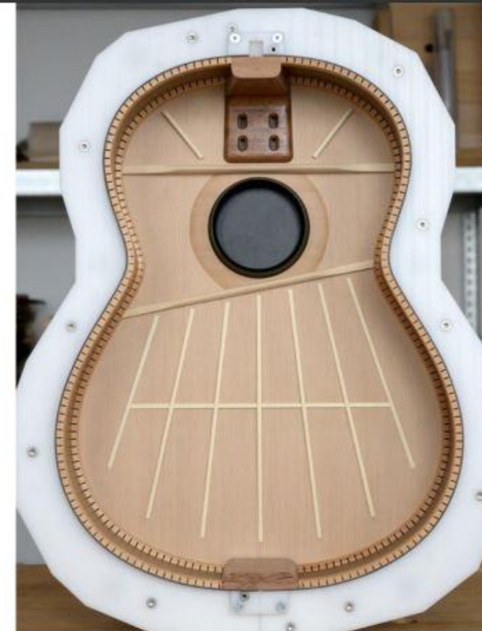
With its bracing completed and "WaveGuide" set in place, the body is ready to be closed with the guitar back.
