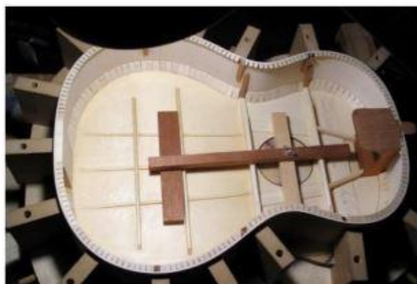
"Concert" model bracing: three-strut vertical fan with two horizontal bars.
