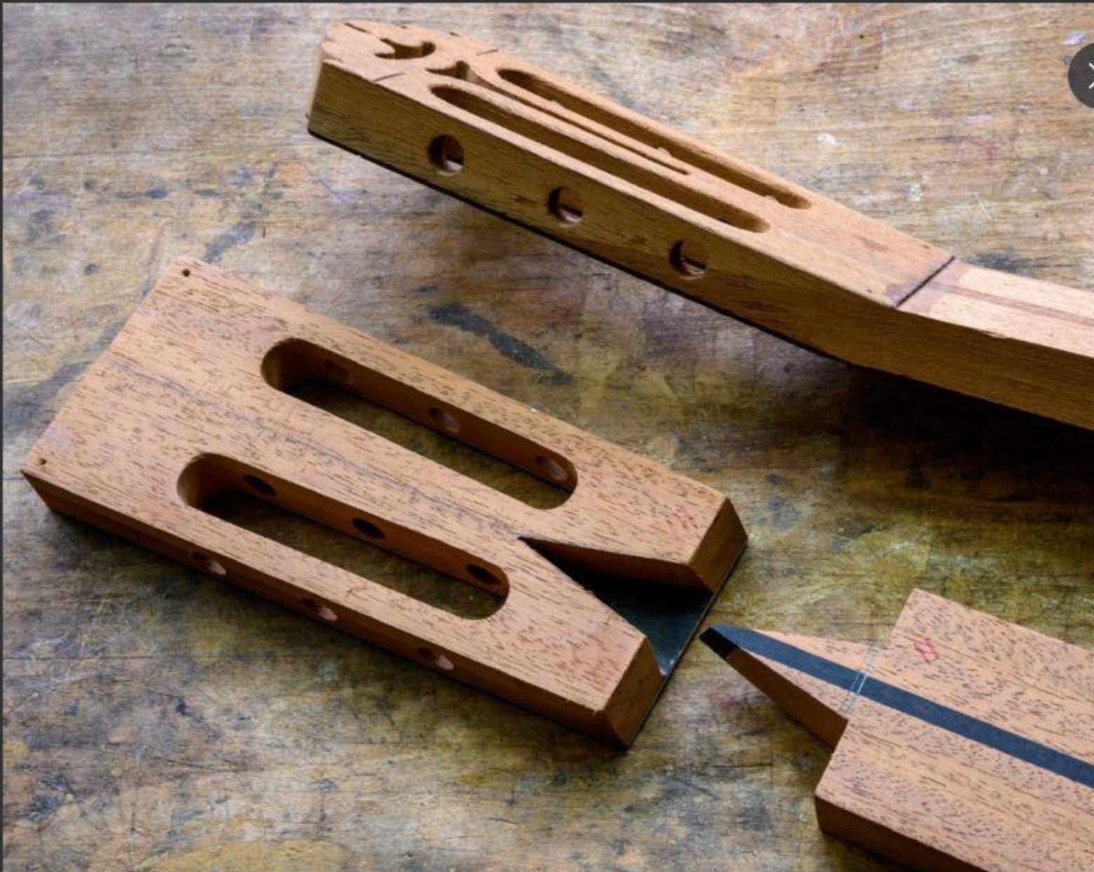
They offer two types of neck/head joint: German-style V-joint, or Spanish-style scarf.
