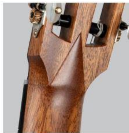
À la Weissgerber: neck/head V-joint and purfling of casein plastic.
