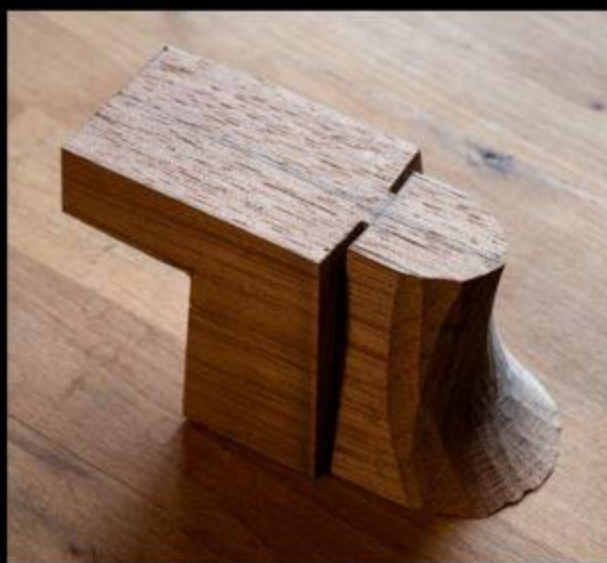
The heel comprises two pieces of Spanish cedar, glued length-wise.
