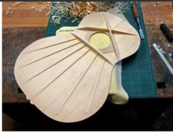
Asymmetrical bracing in the "Elia" model.
