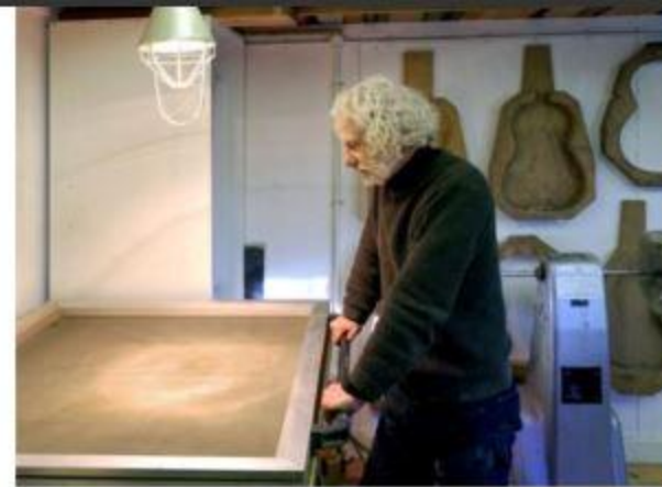
Southwell uses a vacuum press for certain gluing processes.
