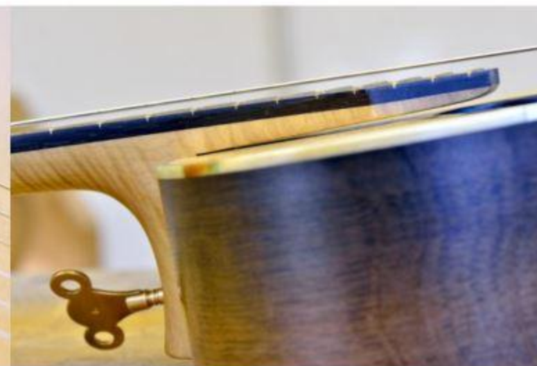
By turning the key, the neck angle is easily adjusted.
