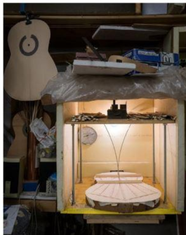
The bracing is glued in a home-made chamber.
