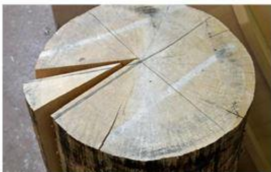
The traditional radial section required for lutherie.
