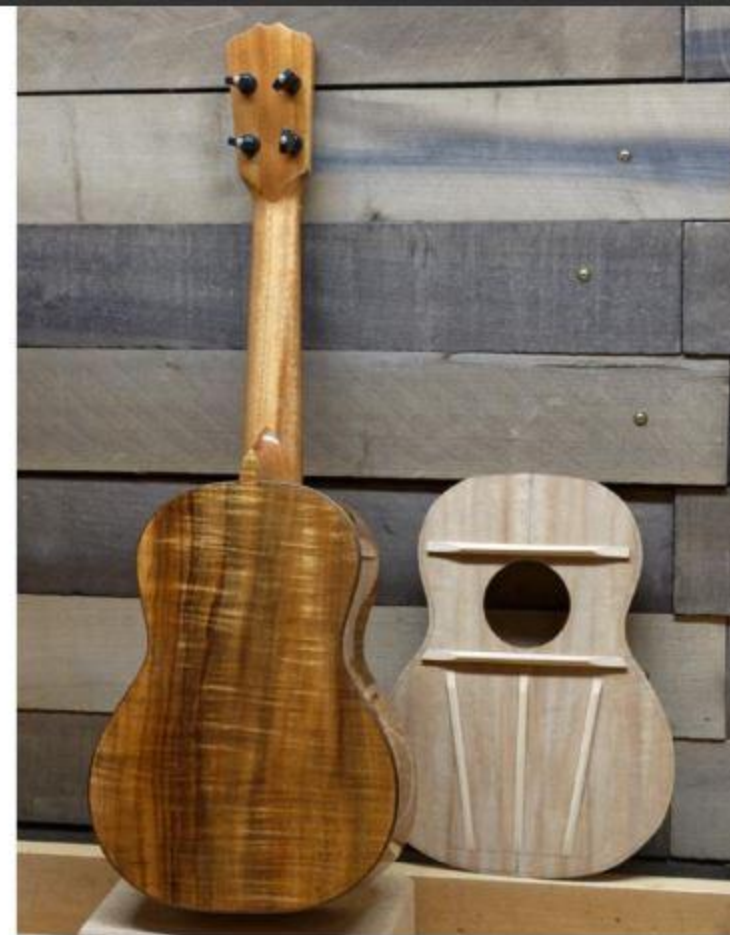
Ukulele made of koa, with three-strut inverse fan bracing.
