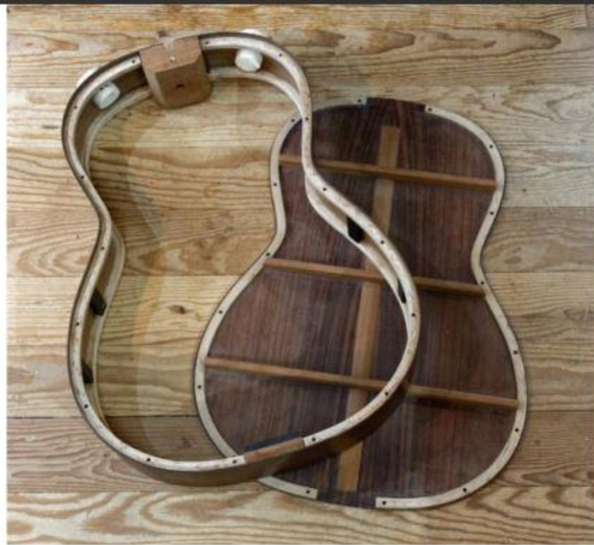
The experimental guitar's back and ribs, which can be reassembled.
