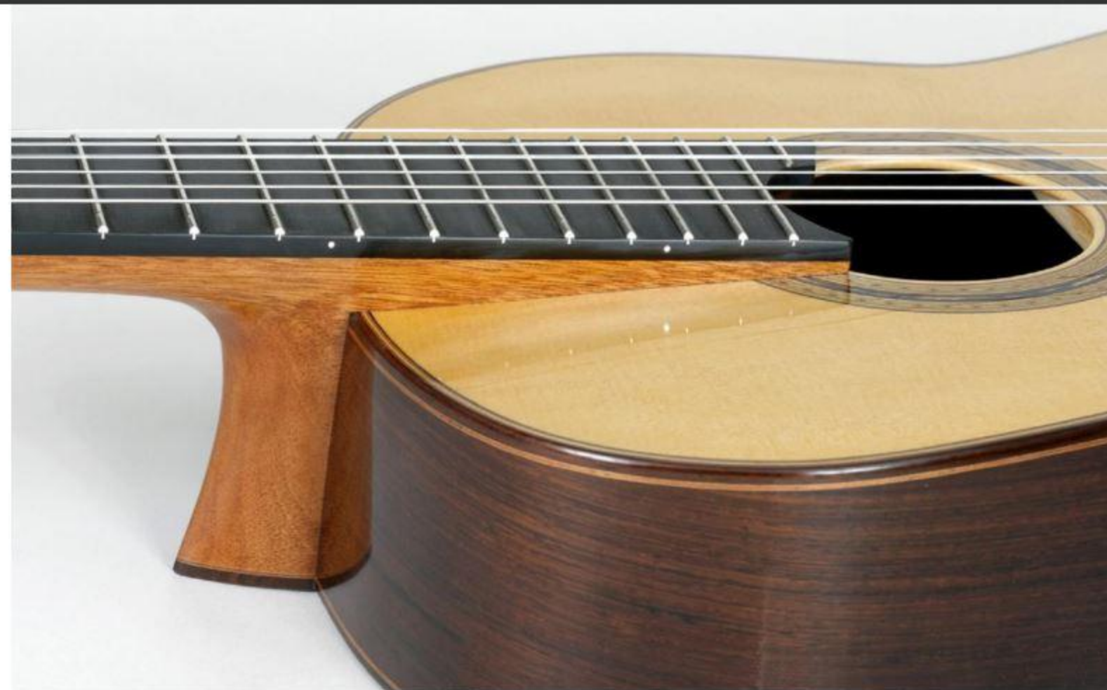
Having a raised fretboard means that the guitar top needs to slope down towards the heel.
