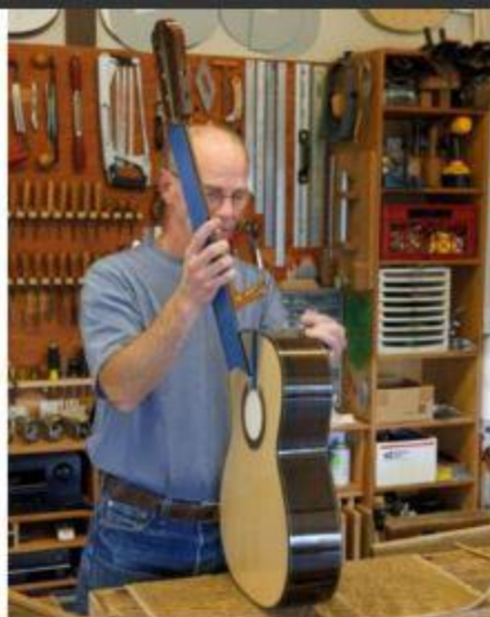
Once the body is finished it's time to glue the neck and screw it on.
