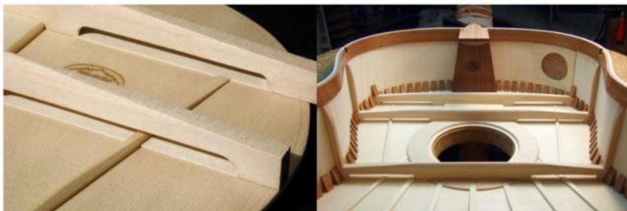
The three soundboard bars are open and reinforced.
