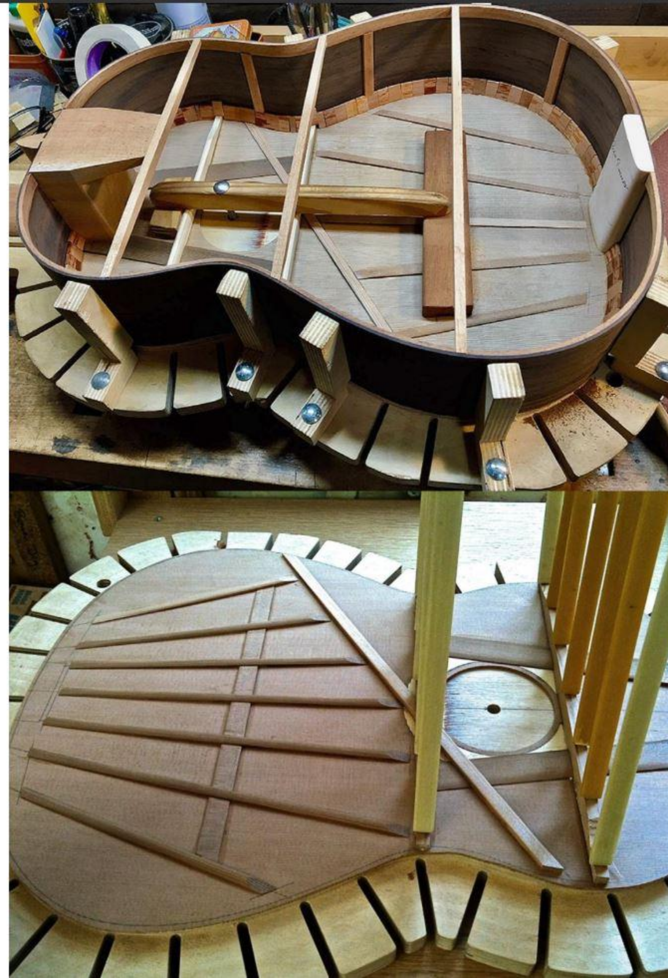
Examples of bracing: five- or seven- strut reverse fans and slanted treble bar.
