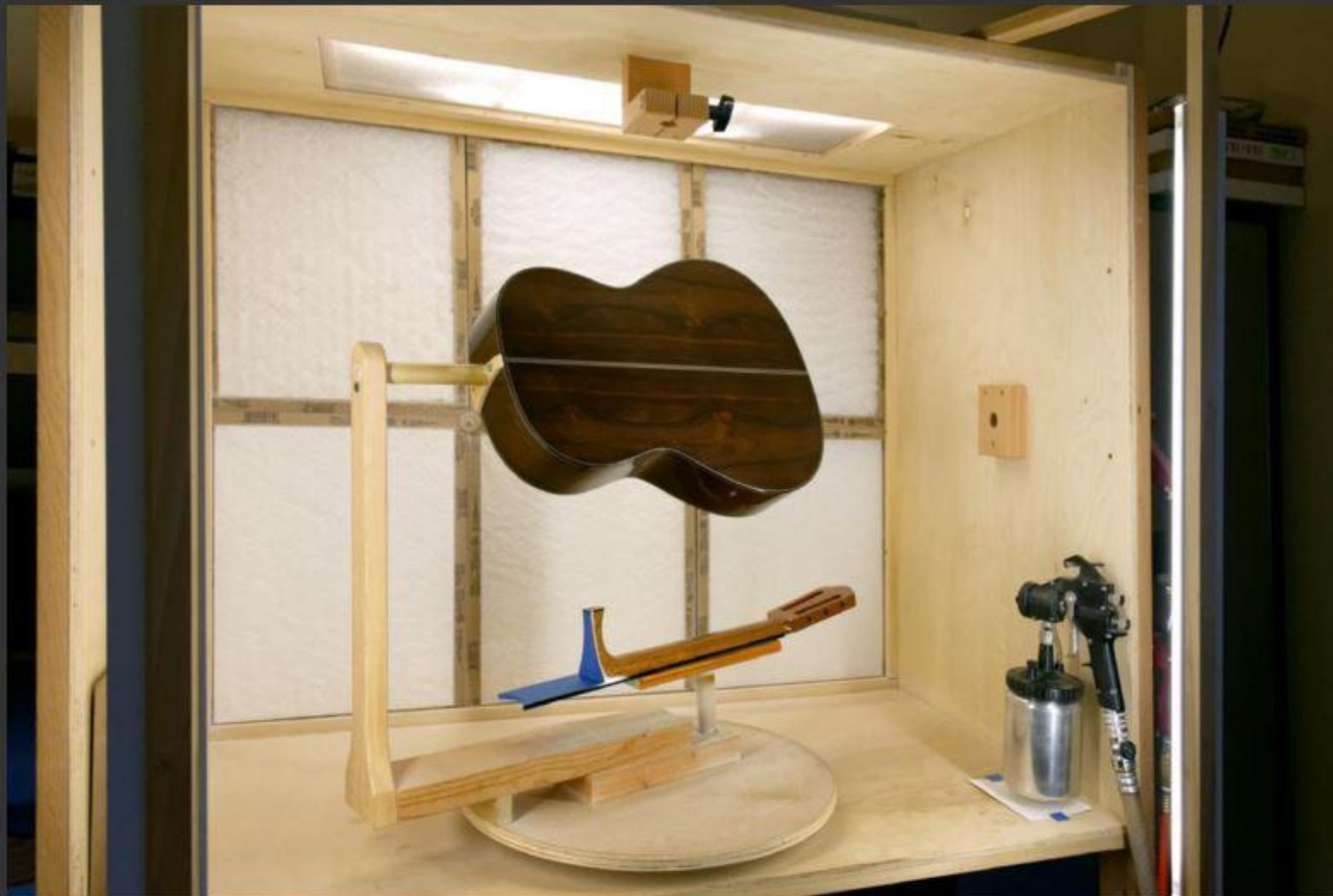
The soundboard is French polished and the back and sides sprayed.
