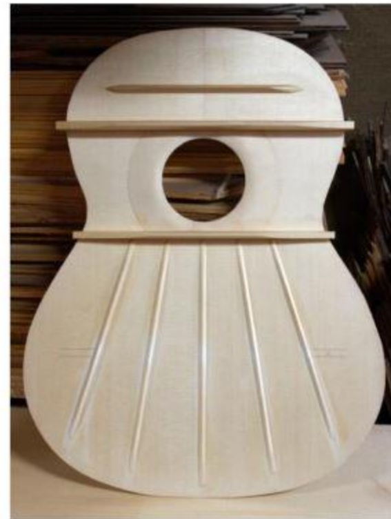
Spruce soundboard under construction.
