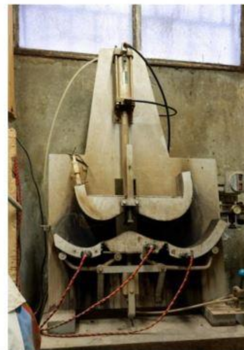
Heated press mould for shaping ribs.
