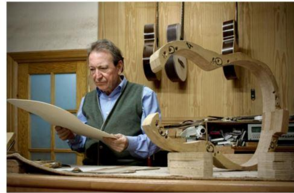
A new mould was needed for the different proportions of the 50 Aniversario.
