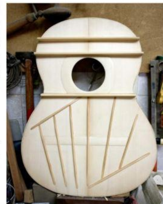
An unfinished soundboard with inverted bracing.
